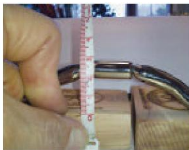
Measurement of a snaffle bit to allow tongue relief. The maximum height of deviation is 30 mm from the lower part of tongue side to the highest part of deviation. The widest part of the deviation must be where the mouthpiece contacts the tongue and must have a minimum width of 30 mm.
